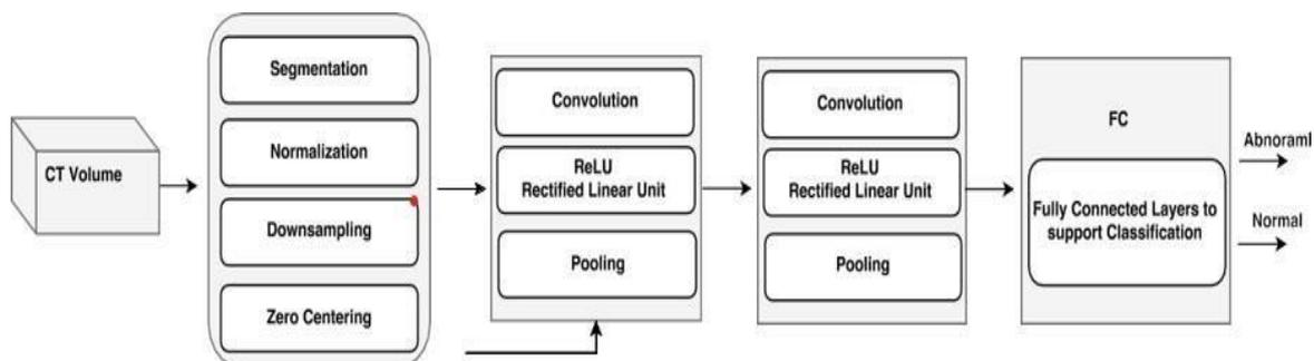
Fig 2. The architecture of a 3D convolutional neural network is present in 3D form [23].
